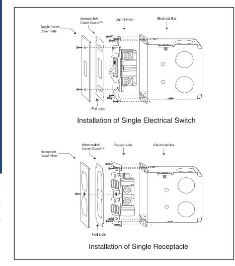
**Step 1** Place aluminum foil side of Metacaulk Cover Guard against inside of electrical face plate.
