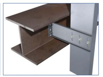
The VertiClip SLB600-10 and 600-12 accommodate an even greater construction tolerance of studs from structure and are now standard products. The VertiClip SLB600-10 is 10" in depth with slot spacing designed for a 6" stud, and the VertiClip SLB600-12 is 12" in depth with slot spacing designed for a 6" stud.
