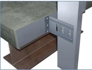
Standard offset of stud from the heel of the clip should not exceed 1.0". Step Bushings and Screws may be installed in the middle and outer slots of SLB600 or 800 to accommodate greater building tolerances. Note that this may affect the F1 and F2 allowable load capacity and may require a row of bridging at a maximum distance of 12" of the connection to resist stud torsional effects. Call TSN Tech Support for test data and recommendations.
