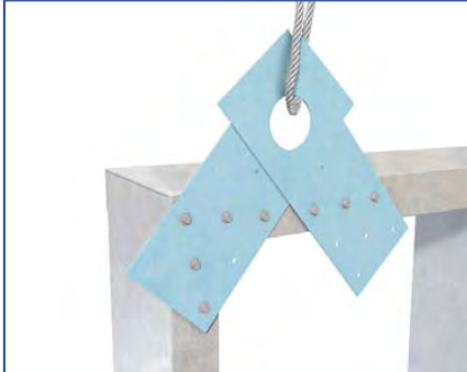
Double Attachment to Wall at End Stud
