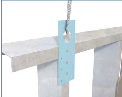
Attachment to Wall at Intermediate Stud
