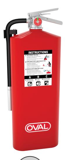
**Application:** Multi-purpose 10 lb. dry chemical fire extinguisher for wall and column mounting. For use on Class A, B and C fires. Not recommended for use on sensitive electronic equipment.
