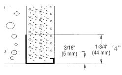
All butt joints, intersections and ends shall be caulked at the time of installation using an elastomeric sealant, such as Plastic Components' Ultra-Tech<sup>™</sup> (PC-ULTW).
