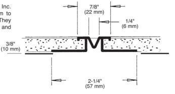
The base coat mesh should be lapped over the top of the perforated flanges and across all butt joints.
