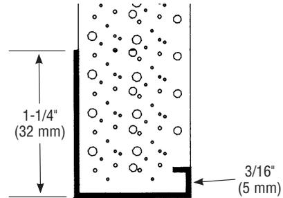
All butt joints, intersections and ends shall be caulked at the time of installation using an elastomeric sealant, such as Plastic Components' Ultra-Tech™ (PC-ULTW).
